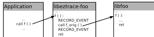
Fig. 1. Instrumentation of the function f with LD_PRELOAD in EZTRACE
