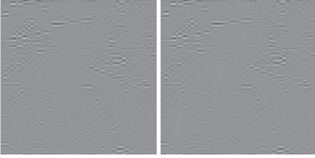
Fig. 22 Estimation of the horizontal detail wavelet atom at level 3. Target u (left) and approximation \lambda\alpha * h^1 * \dots * h^K (right). NRE = 0.68
