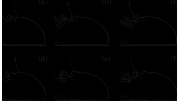
Fig. 4 Snapshots of the head at different time instants obtained with the finite-volume method ( Re = 10^4 , Sc \rightarrow \infty ): a–c 1,248 \times 240 grid and d–f 1,664 \times 320 grid. The time difference between snapshots is constant and the same for both grids ( \Delta \tilde{t} = 0.56 ). The values of the plotted contours are \tilde{\rho} = 0.05, 0.275, 0.5, 0.725 and 0.95 . Images are vertically stretched by a factor 2. Note that the position of the current’s front at a given time instance is identical for all the spatial resolutions
