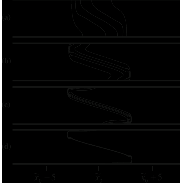
Fig. 5 Contours of \tilde{\rho} at \tilde{t} = 12.7 ( Re = 10^2 ). Results for a Sc = 1 , b Sc = 10 , c Sc = 10^2 and d Sc \rightarrow \infty . Frames a to c are from the spectral code for which the grid resolution is 1,024 \times 80 on a 32H \times H over-all domain. Frame d is from the finite-volume code for which the grid resolution is 1,600 \times 160 on a 25H \times H domain. The values of the plotted contours are \tilde{\rho} = 0.05 - 0.275 - 0.5 - 0.725 - 0.95 . Images are vertically stretched by a factor 3.33
