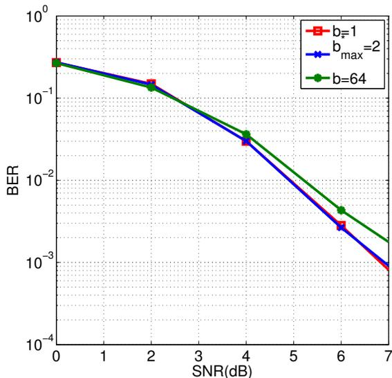
Fig. 4: Bit Error Rate for an OFDMA system with CFO for the scenario  $N_p = 128$ ,  $N_u = 2$  and  $L = 32$ . The CFO of each user is independently uniformly generated in  $[0, 0.01]$ . The optimal block-sizes are  $b^* \in \beta^* = \{1, 2\}$ .
