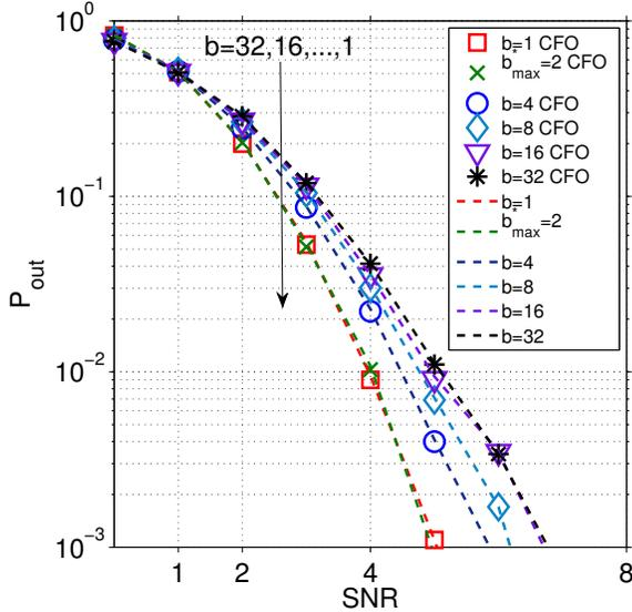
Fig. 3: Outage probability for an OFDMA system without CFO (dashed lines, appearing in decreasing order of block-size from up to down) and with CFO (marker lines) for the scenario  $N_p = 64$ ,  $N_u = 2$  and  $L = 16$ . The CFO of each user is independently uniformly generated in  $[0, 0.01]$ . The optimal block-sizes are  $b^* \in \beta^* = \{1, 2\}$ .
