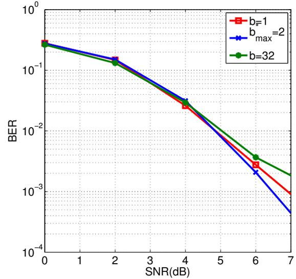
Fig. 5: Bit Error Rate for an OFDMA system with CFO for the scenario  $N_p = 128$ ,  $N_u = 2$  and  $L = 32$ . The CFO of each user is independently uniformly generated in  $[0, 0.03]$ . The optimal block-size is  $b_{max}^* = 2$ .
