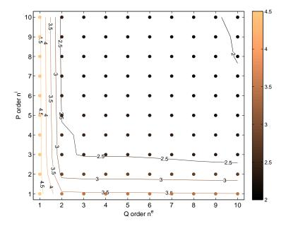
**Figure 3.** Contour and scatter plot of  $log(J(u_{opt}))$  as a function of the maximum order of the associated Legendre functions of first kind  $n^i$  and second kind  $n^e$  used for the representation of the flux.
