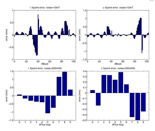
**Figure 7.** Error introduced on X-point position reconstruction by adding a 10 mT offset on a single Booil measurement or a 200 mWb offset on a single flux loop measurement.
