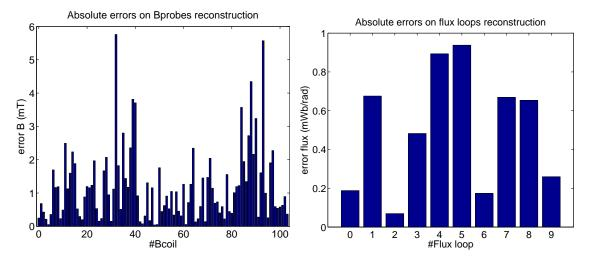
**Figure 5.** Comparison between measured and reconstructed values for WEST case 1 using  $(n^e = 4, n^i = 4)$ .
