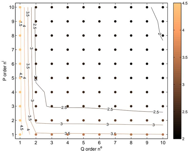
**Figure 3.** Contour and scatter plot of  $\log(J(u_{opt}))$  as a function of the maximum order of the associated Legendre functions of first kind  $n^i$  and second kind  $n^e$  used for the representation of the flux.
