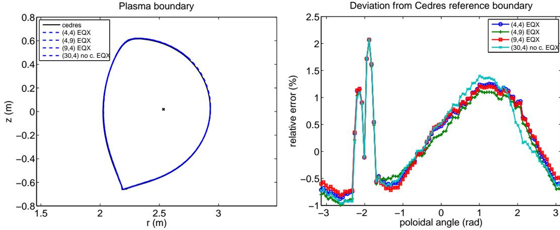
**Figure 6.** Left: Plasma boundaries. Boundaries computed by Equinox (EQX) with  $(n^e = 4, n^i = 4)$  or  $(n^e = 9, n^i = 4)$  and  $(n^e = 30, n^i = 4)$  without any PF coils modelization (no c.) are almost superimposed with the reference boundary computed with Cedres++. The boundary computed with Equinox  $(n^e = 4, n^i = 9)$  does not show any irregularities.
