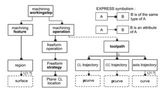
Figure 6: Free-form machining with STEP-NC.
