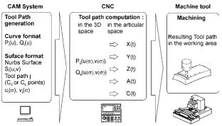
Figure 2: Method for curve machining.
