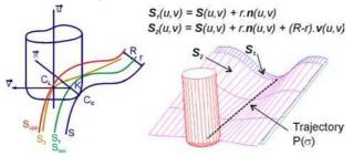
Figure 4: Definition of the surface format in 5 axes.
