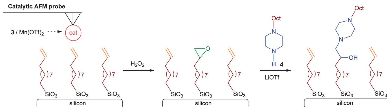
Scheme 1 Local alkene SAM epoxidation by a catalytic AFM probe, loaded with \text{Mn}(\text{OTf})_2 /ligand 3 and \text{H}_2\text{O}_2 as co-oxidant in acetonitrile, followed by AFM-free nucleophilic ring-opening reaction of epoxide sites with amine 4 .
