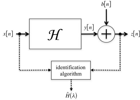
Figure 3. Non-parametric identification of a LTI system  $\mathcal{H}$  in the frequency domain.
