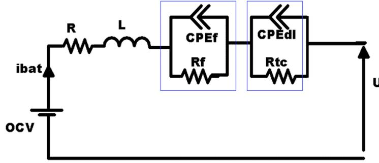
Figure 4. Equivalent electrical circuit (adapted Randles model) of a graphite/LiFePO<sub>4</sub> battery.
