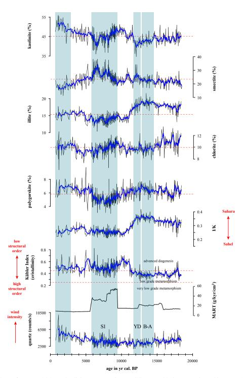
**Fig. 2.** Clay mineralogy of core MD04-2797: kaolinite (%), smectite (%), illite (%), chlorite (%), palygorskite (%), I/K: illite to kaolinite ratio, Kübler index (crystallinity), (MART) Terrigenous Mass Accumulation Rates (g kyr<sup>-1</sup> cm<sup>-2</sup>) and quartz content (counts/s) for the last 20 000 yr. B–A = Bølling–Allerød, YD = Younger Dryas, S1 = sapropel S1 (Mercone et al., 2000).
