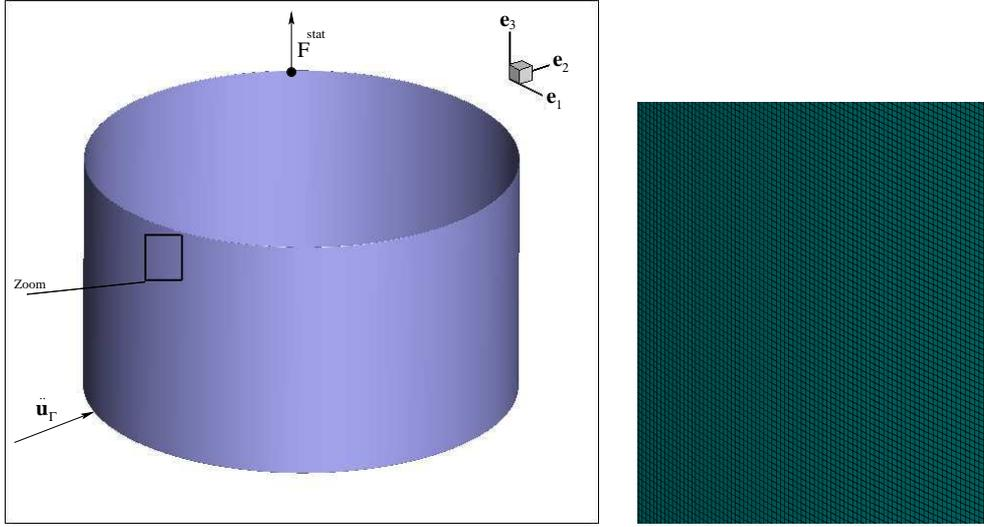
Figure 1: Left part: 3D representation of the cylindrical shell with boundary conditions ( $\circ$  denotes the only free node of the upper bound of the cylindrical shell, corresponding to the node  $obs$ ). Right part : zoom of the mesh.
