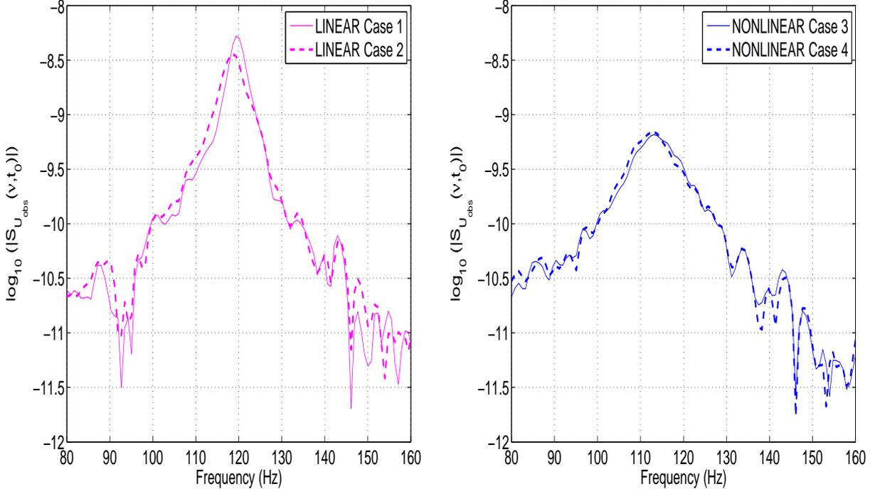
Figure 5: Graphs of  $\nu \mapsto \log_{10}(|S_{U_{obs}}(\nu, t_0)|)$  without and with random uncertainties (thin line and thick dashed line): linear case (left graph) and nonlinear case (right graph).
