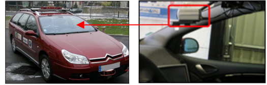
Figure 7: Carmen: The experimental vehicle of the Heudiasyc Laboratory with the monocular vision system.
