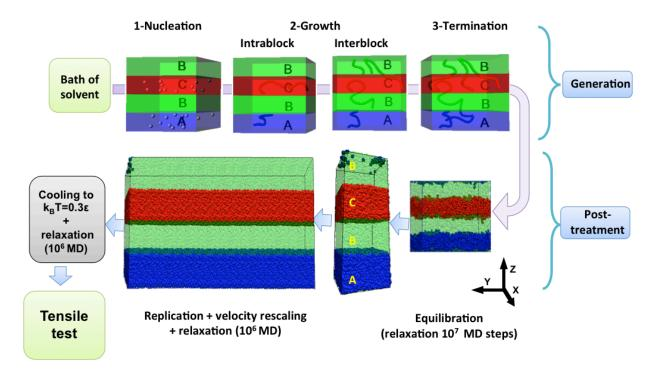
Figure 2: Schematic description of the generation and the post treatment process. Starting from a bath of monomers ("solvent"), the Radical Like Polymerization routine will transform the single disconnected beads to entangled chains. The polymerization occurs in 4 blocs A, B, C and B. The resulting chains are shared between three successive blocks A, B and C. LJ interaction energies are chosen so that a perfect segregation of the blocks is ensured at low temperature.
