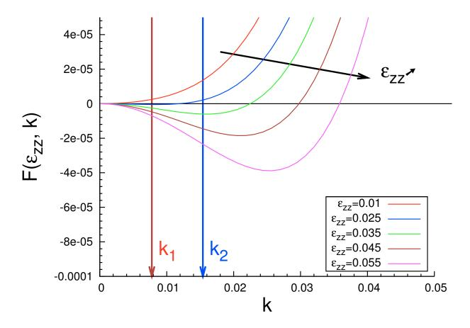
Figure 5: Evolution of  $F(\varepsilon_{zz},k)$  (see equations 15 and 17) for different levels of strain, the two arrows denote the wavevectors  $k_1=2\pi/L_y$  and  $k_2=4\pi/L_y$ .
