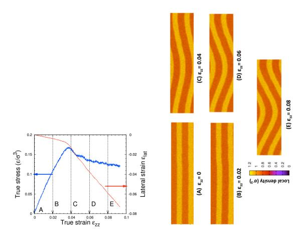
Figure 7: Low strain rate tensile test: the upper panel shows the stress strain curve for the same sample illustrated in figure 3, together with the evolution of s the lateral strain. In this case, the yield corresponds to the onset of the buckling. The arrows indicate the strain levels at which the snapshots presented in the lower panel are taken. Cavities are completely absent from the rubbery phase.
