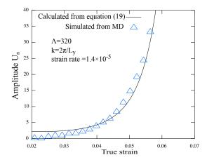
Figure 12: Comparison between the measured values of buckling amplitude (disconnected symbols) and the value calculated from equation 9 (full lines) for the largest sample  $L_y = 787.2\sigma$ . The left panel corresponds to fundamental mode  $k = \frac{2\pi}{L_y}$  observed at low strain rate, whereas the right panel corresponds to the second mode  $k = \frac{4\pi}{L_y}$  at high strain rate. The value of  $\Lambda$  taken here corresponds to the best fit of the measured amplitude.
