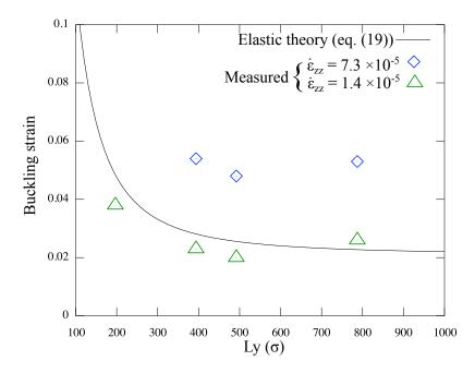
Figure 10: Comparison between the buckling strain values predicted from the elastic theory (19) and the one measured from MD simulations for all samples at two strain rates  $7.3 \times 10^{-5}$  and  $1.4 \times 10^{-5}$ .
