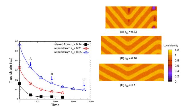
Figure 11: Left: relaxation of the strain in a system unloaded instantaneously after being deformed to the strains indicated in the figure. Right: snapshots of the relaxing configuration (density field) at the three states indicated by A,B, C in the left panel.
