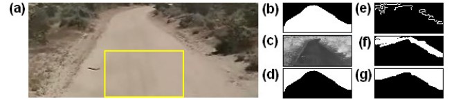
Fig. 3 – (a) Original image after sky removal and its Otsu's result in (b); (c) negated image and its Otsu's result in (d); (e) Canny edge detection result; (f) Hough transform result; (g) a single mass in the image (f).
