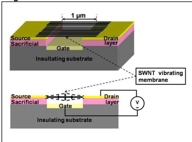
Fig. 1: Schematic view of SWNT-based capacitive ultrasonic transducer
