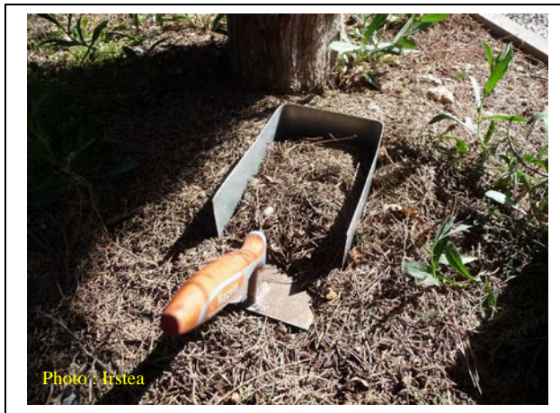
Fig. 2: Sampling of undisturbed cypress litter
