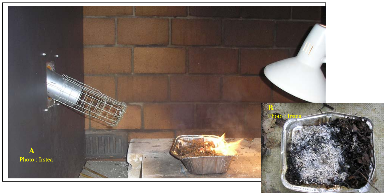
Fig. 3: The burning device used for the flammability experiments (A) and a top view of a burned sample showing the results of the flame spread (B). Domestic fan provides a 9.8 kmh -1 wind.
