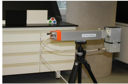
Figure 2. Image acquisition setup with white and black reference plates.
