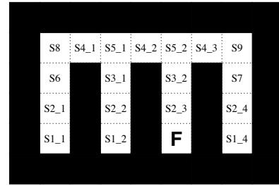
Figure 4: The Maze10 environment. **F** represents the goal to reach (food) from any cell of the maze; a few cells are unambiguous ( $S_i$ ) but in the other ones the same perceptual situations may require either similar actions or different ones (e.g. go north in  $S_{2\_ \{1,2,4\}}$  but go south in  $S_{2\_3}$ )
