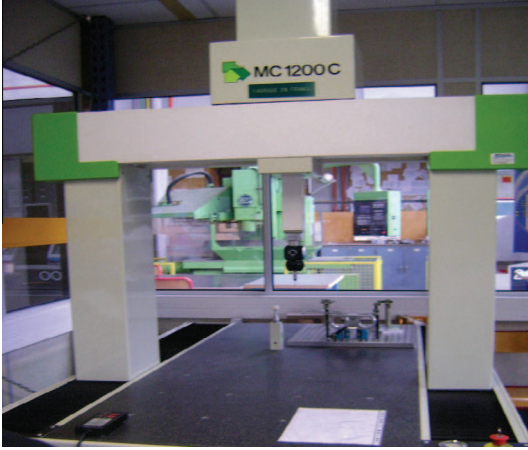
Fig. 5. Three-dimensional measuring machine "MC 1200C".
