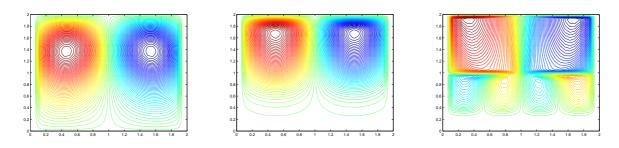
Figure 2: Stationary convective regimes. Level lines of the stream function for  $F_K = 1$ ,  $R_p = 100$  (left), for  $F_K = 1$ ,  $R_p = 1000$  (middle) and for  $F_K = 3.2$ ,  $R_p = 1000$  (right).
