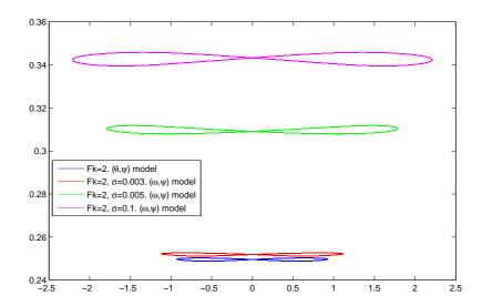
Figure 7: Mean of temperature as function of mean of stream function for  $R_p = 4 \times 10^3$  and for different values of  $\sigma$ . Solution of the complete Darcy's law converges to the solution under quasi-stationary approximation as  $\sigma$  decreases.
