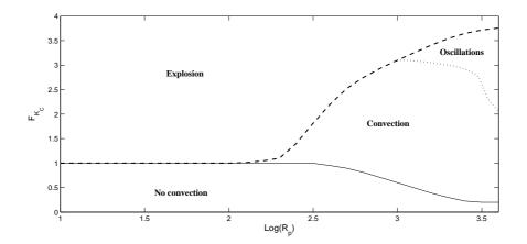
Figure 1: Numerical simulations reveal four different regions in the parameter plane  $(R_p, F_K)$ . In the lower region, there are stationary regimes without convection. In the upper region, they do not exist and solution blows up. In the intermediate region from the right, the solution remains bounded (no explosion). It can be stationary or oscillating with convection.
