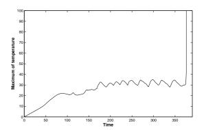
Figure 6: Maximum of the stream function (left) and of the temperature (right) as functions of time for  $R_p = 4 \times 10^3$  and for  $F_K = 3.757$ .
