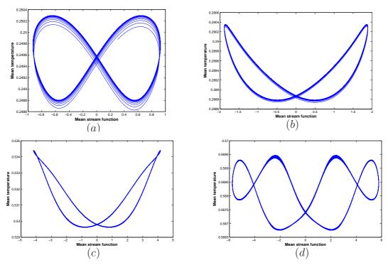
Figure 5: Oscillating convective regimes. Mean of temperature as function of the mean value of the stream function for  $R_p = 4 \times 10^3$  and for different values of  $F_K$ ,  $(a)F_K = 2$ ,  $(b)F_K = 2.2$ ,  $(c)F_K = 3.5$ ,  $(d)F_K = 3.7$ .
