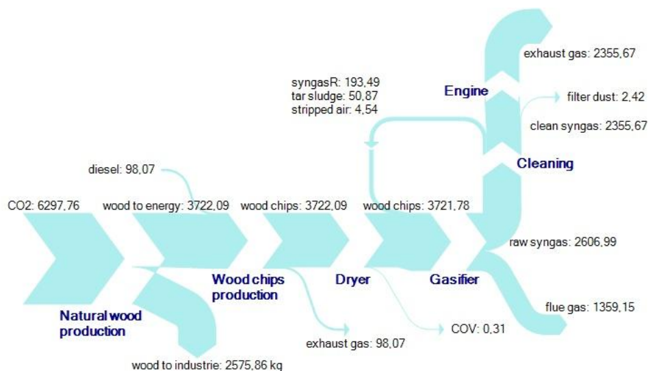
Fig. 5: Carbon mass flow rate (kg/h) along the biomass to energy chain based on a 10MWelec gasification unit
