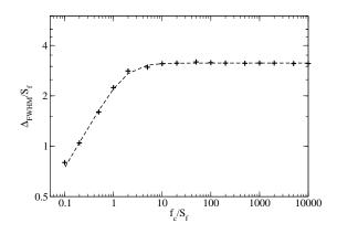
FIGURE 17. Comparison of the laser FWHM (crosses) with the empirical formula (dashed line) given in Eq. (D1).
