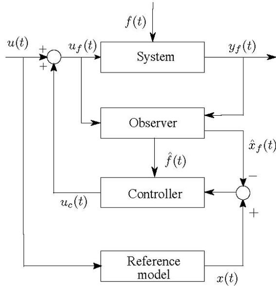
Fig. 1. Tracking fault tolerant controller design scheme
