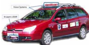
Figure 1: Experimental Vehicle CARMEN with its 4-Layers lidar and Vision Systems
