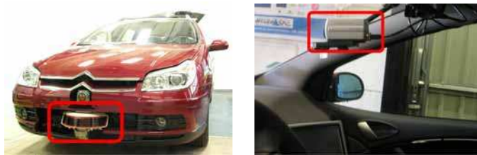
Figure 11: CARMEN experimental platform, showing the relative locations of the sensors
