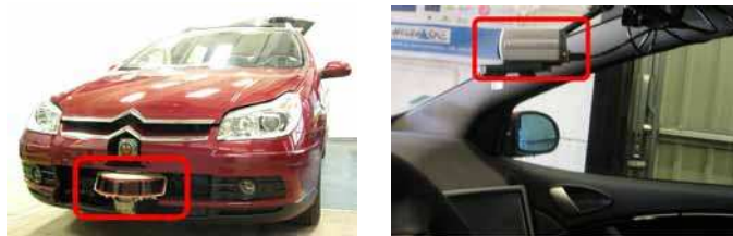
Figure 11: CARMEN experimental platform, showing the relative locations of the sensors
