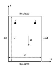
Figure 1: Differentially heated cavity with insulated horizontal walls and constant temperature vertical walls. The aspect ratio is A=H/W. Points 1 and 2, respectively in  $(x_1,y_1)$  and  $(x_2,y_2)$ , are time history points.
