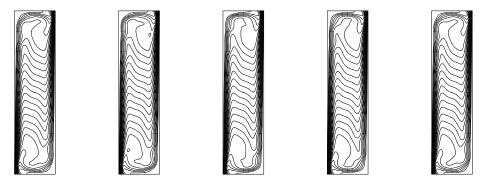
Figure 3: Iso-lines of temperature (difference between two iso-lines:  $\delta T = 3.84 \times 10^{-2}$ ) over one period  $\tau$ . Left to right  $t = 0, \tau/4, \tau/2, 3\tau/4, \tau$ .  $Ra = 3.4 \times 10^5, Pr = 0.71, Ma = 10^{-1}$  and  $N_x \times N_y = 301 \times 2401$ .
