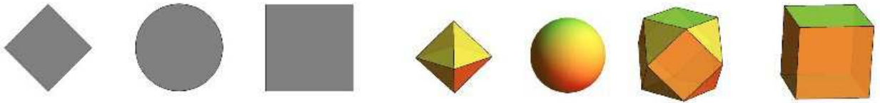
Figure 1: Structuring elements in 2D for the norms [\cdot]_1 = \ell^1 , \ell^2 , [\cdot]_0 = \ell^\infty and in 3D for the norms [\cdot]_2 = \ell^1 (octahedron), \ell^2 , [\cdot]_1 (cuboctahedron), [\cdot]_0 = \ell^\infty .
