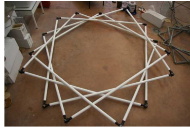
Figure 22: Physical model for a foldable tensegrity ring
