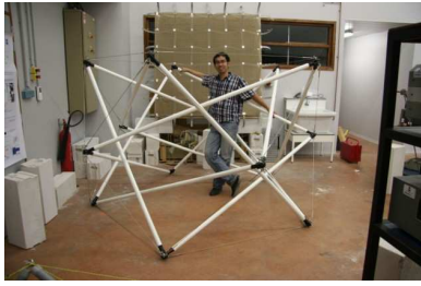
Figure 22: Physical model for a foldable tensegrity ring
