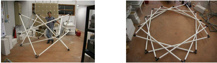
Figure 22: Physical model for a foldable tensegrity ring
