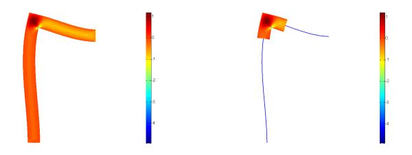
Figure 25: A plane frame analysis: comparison of  $\sigma_{xy}$  contour plot obtained with solid model (left) and solid-beam model (right).
