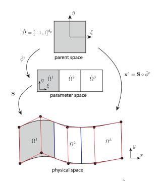
Figure 5: Diagrammatic interpretation of mappings from parent space  $(\hat{\Omega})$  through parametric space  $(\hat{\Omega})$  to physical space  $(\Omega)$ . The parent space is where numerical quadrature rules are defined.
