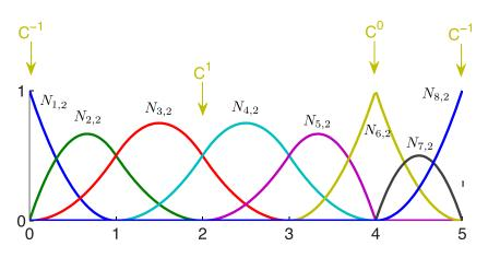
Figure 4: Quadratic B-spline basis functions defined for the open, non-uniform knot vector  $\Xi = \{0, 0, 0, 1, 2, 3, 4, 4, 5, 5, 5\}$ . Note the flexibility in the construction of basis functions with varying degrees of regularity.
