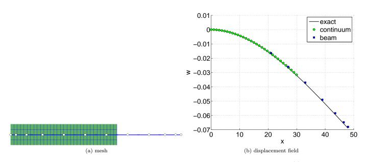
Figure 22: Mixed dimensional analysis of the Timoshenko beam with non-conforming coupling: (a)  $32 \times 4$  Q4 elements and 8 quartic (p = 4) beam elements and (b) displacement field.
