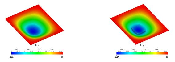
Figure 33: Square plate enriched by a solid: transverse displacement plot on deformed configurations of plate model (left) and solid-plate model (right).
