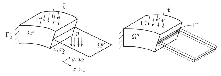
Figure 3: Coupling of a three dimensional solid and a plate.
