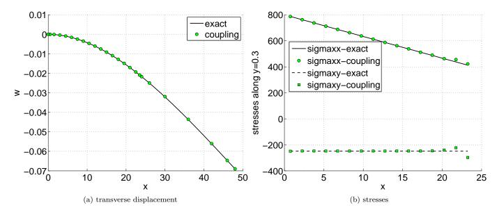
Figure 17: Mixed dimensional analysis of the Timoshenko beam with B-spline elements: comparison of numerical solution and exact solution.
