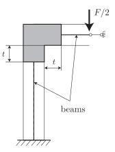
Figure 24: A plane frame analysis: solid-beam model.
