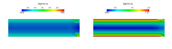
Figure 19: Mixed dimensional analysis of the Timoshenko beam with B-spline elements: numerical shear stresses with  $\nu = 0.3$  and  $\nu = 0.0$ .
