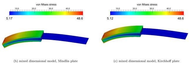
Figure 29: Cantilever beam subjects to an end shear force
