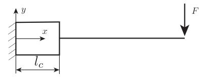
Figure 14: Timoshenko beam: mixed continuum-beam model.
