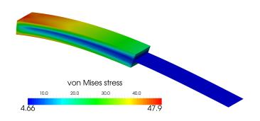
Figure 31: Cantilever beam subjects to an end shear force: von Mises stress distribution.
