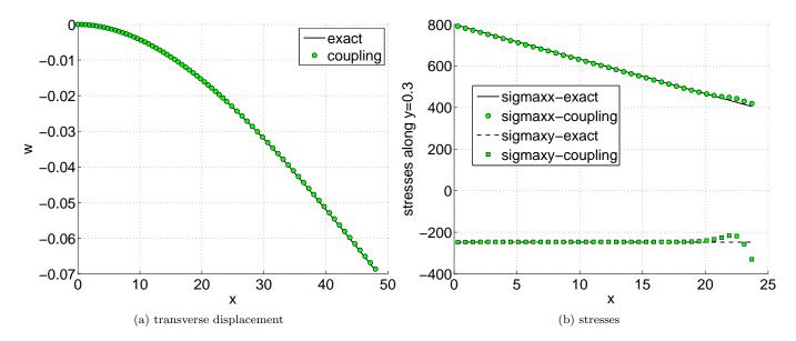
Figure 15: Mixed dimensional analysis of the Timoshenko beam: comparison of numerical solution and exact solution.
