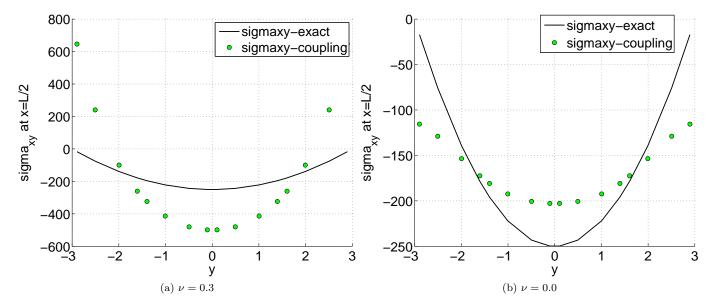
Figure 20: Mixed dimensional analysis of the Timoshenko beam with B-spline elements: numerical shear stresses along the coupling interface with  $\nu = 0.3$  and  $\nu = 0.0$ . The distribution of the shear stress with  $\nu = 0.3$  is very similar to the result presented in [38] that uses the MPC (cf. Figure 18 of the referred paper).
