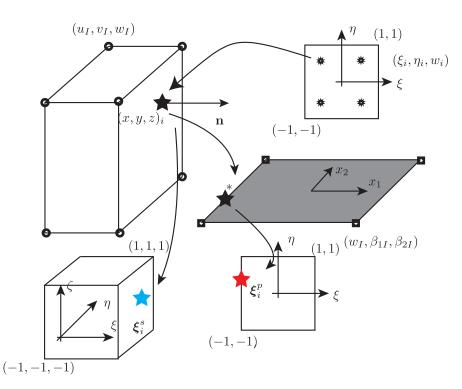
Figure 9: Coupling a plate and a 3D continuum using a Nitsche based method: determination of Gauss points for evaluating the coupling terms.
