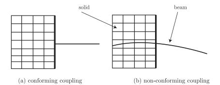
Figure 1: Solid-structure coupling: (a) conforming coupling and (b) non-conforming coupling. The bold lines represent the coupling line/surface.
