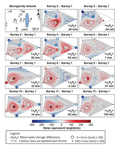
**Figure 8.** Weekly maps of the residual contribution of the vadose zone. The MDg values were corrected for the pond and aquifer effects and converted into water equivalent heights. Positive values indicate that the water storage in the vadose zone is above the mean of the whole gravity network, and conversely for negative values. The dates of the beginning and end of each survey are listed in Table 2. The marks on *x* and *y* axes represent 50 m increments.
