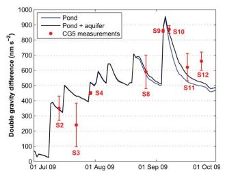
**Figure 4.** Comparison of the relative gravity signal measured at the pond station (red dots) with two models, taking into account the variation in the pond water level (blue line) or in the pond and groundwater levels table (black line). The aquifer model considers a heterogeneous distribution of porosities derived from MRS (Figure 6). The number X of the survey is indicated by SX beside each measurement point.
