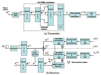
Fig. 2. SC-FDMA transmission scheme
