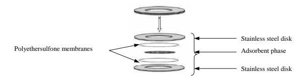
Fig. 1: Schematic illustration of a POCIS device.
