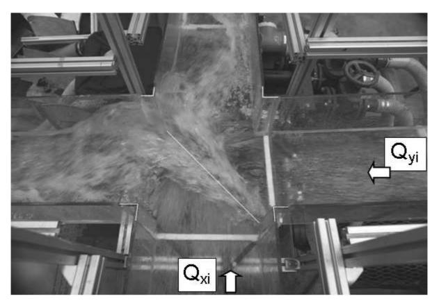
Figure 1 : Aerial photograph of Case 1 flow. The continuous white line is the main diagonal of the square intersection.
