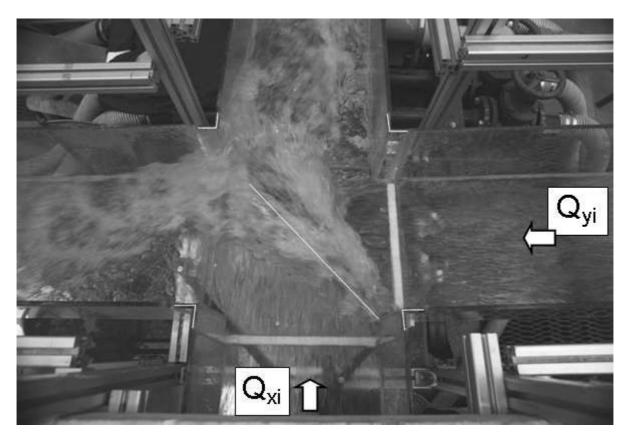
Figure 2 : Aerial photograph of Case 2 flow. The continuous white line is the main diagonal of the square intersection.
