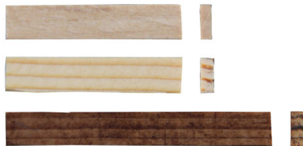
1 Top view and cross-section of specimens for three-point bending tests in DMA equipment: from top to bottom, beech and spruce before thermal modification/DMA with length of 30 mm and spruce after thermal modification/DMA with length of 45 mm; nominal cross-section of all specimens was width w \times thickness t=6 \times 2 mm
