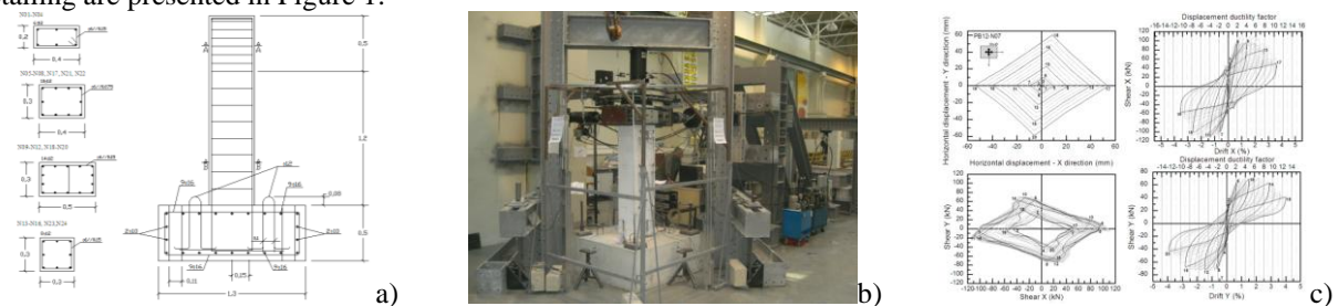
Figure 1: Testing setup: a) RC column specimen dimensions and reinforcement detailing; b) General view; c) Global results of rectangular column PB12-N07 for rhombus load path
