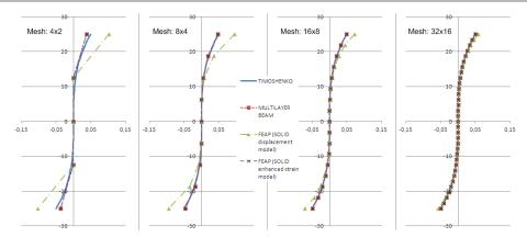
Figure 2: A comparison between the warped cross-section of the left-hand end of the beam according to the theory of elasticity and the linear-piecewise cross-sections obtained by the multi-layer beam model and the two-dimensional finite element models for different meshes
