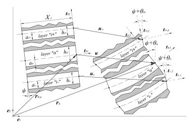
Figure 1: Undeformed and deformed state of the multilayer composite beam
