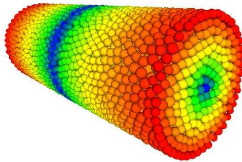
Figure 1: Exemple of discrete domain created with the *cooker* program and drawn by the *gddviewer* program. The discrete cylindrical sample is loaded in a torsion mode where an equal and opposite torque is applied to the faces of the sample. The color scale corresponds to the norm of the discrete element displacements.
