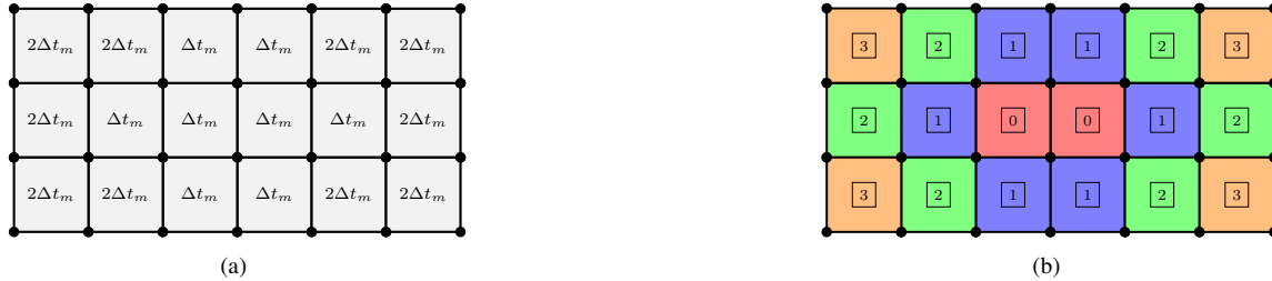
Figure 1: Element-wise stable time steps (a) and multirate groups with associated tags (b).
