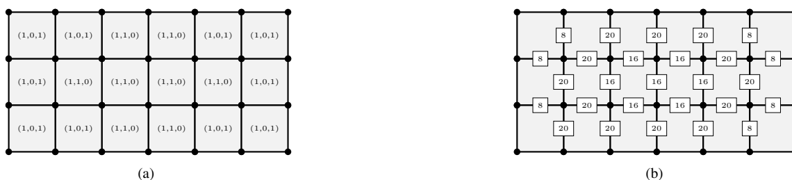
Figure 3: Associated binary vectors for elements (a) and scalar weights for faces (b) for MeTiS partitioner.
