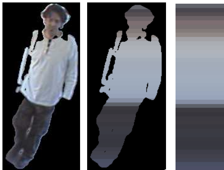
Figure 3: Colour-position signature (left to right: silhouette extraction, colour-position signature extraction, signature vector).
