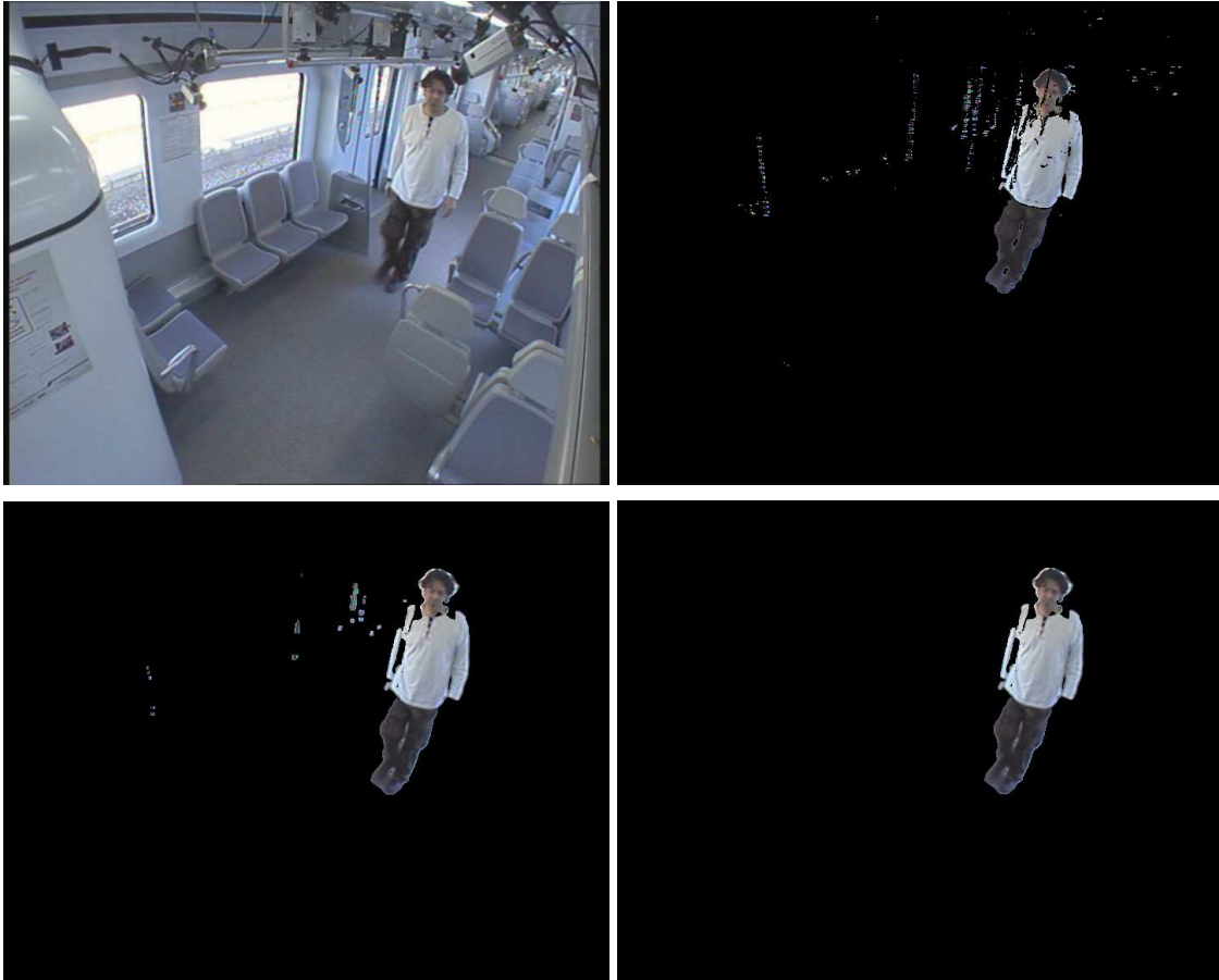
Figure 2: Silhouette extraction (left to right, top to bottom: original frame, background subtraction by codebook algorithm, result obtained by morphological operators, final silhouette after applying CCL algorithm).
