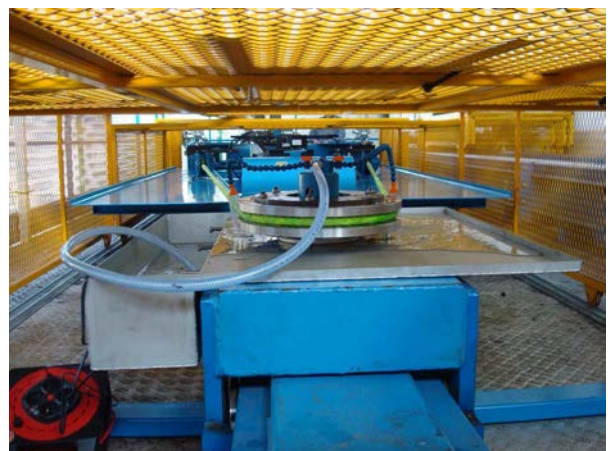
Figure 3. CBOS test machine, showing water spray device.
