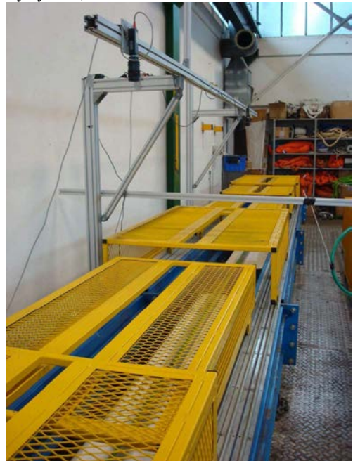
Figure 2. 1000 kN tensile test frame, showing video extensometer system mounted above machine.
