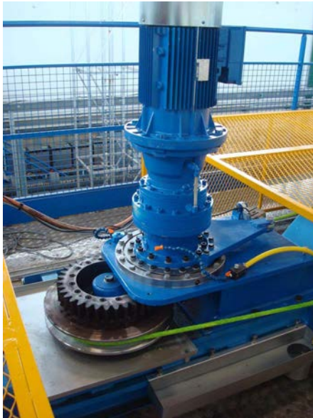
Figure 4. Device allowing known torque to be applied to sheave
