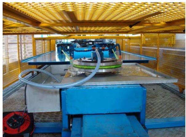
Figure 3. CBOS test machine, showing water spray device.
