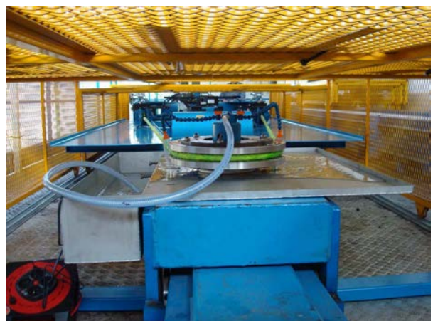
Figure 3. CBOS test machine, showing water spray device.
