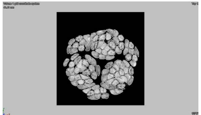
Figure 7. Tomography image of section through braided rope sample before testing.
