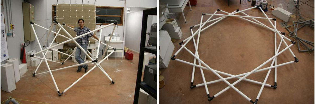
Fig. 25 Physical model for a tensegrity ring (unfolded and folded states)
