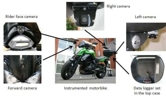
Figure 3: Camera instrumentation mounted on one of the participant's motorcycle
