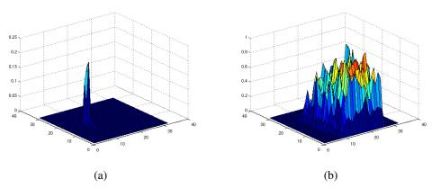
Figure 10. Grid-wise RNCC of AES layouts for with 95% core utilization rate for Original layout and Infected Layout with (a) 1 AND gate, (b) 128 AND gate.
