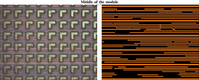
Figure 4. Picture (*left hand side*) and GDSII layout (*right hand side* – M6 in orange for Middle and Side of the module, M5 in yellow for Side of the module) of an AES-128 cryptographic accelerator (area size:  $67 \mu m \times 60 \mu m$ )
