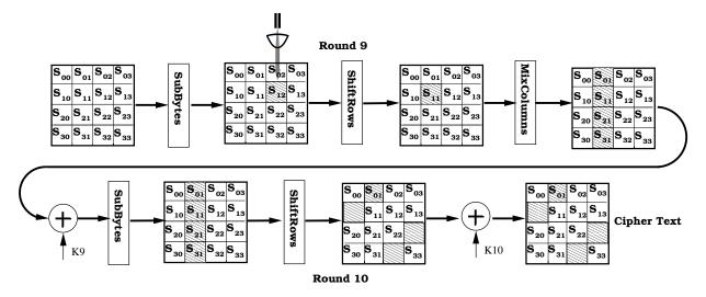
Figure 2. Effect of a fault in last but one round of AES-128.
