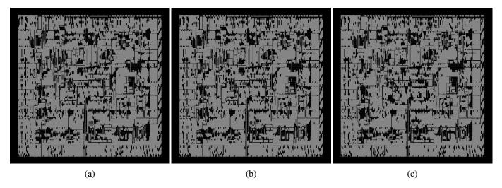
Figure 6. 6th metal layer AES layouts (1200  $\mu$ m × 1200  $\mu$ m) with 50% core utilization rate for (a) Original AES, (b) AES with 1 AND gate HTH, (c) AES with 128 AND gate HTH
