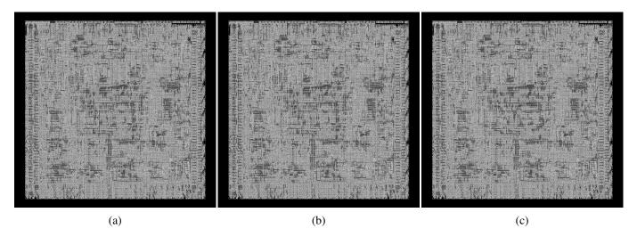
Figure 7. AES layouts (1200  $\mu$ m  $\times$  1200  $\mu$ m) with 50% core utilization rate for (a) Original AES, (b) AES with 1 AND gate HTH, (c) AES with 128 AND gate HTH
