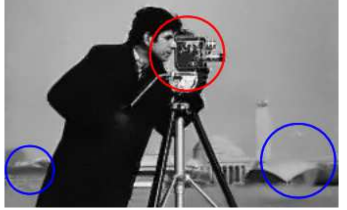
Fig. 1. Illustration of the defaults of the NL-means : the rare patch effect (red circle) can be observed around the head and the camera, while the patch jittering effect (blue circles) can be observed on the background.
