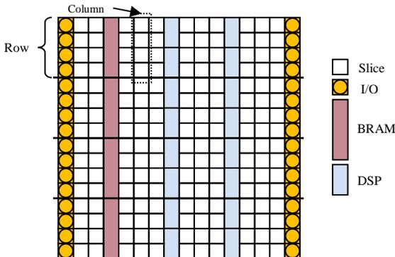
Figure 1. Example of resources repartition on Xilinx FPGA.
