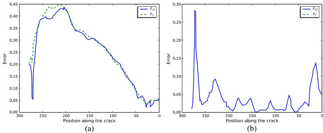
Figure 13. Error indicator on the crack opening (fine mesh, the notch is on the left of the curve): (a) strong approach and (b) weak approach.  $\epsilon_I$  stands for definition (17) of the error, and  $\epsilon_D$  stands for the error of the estimated opening with respect to the direct calculation of the opening.
