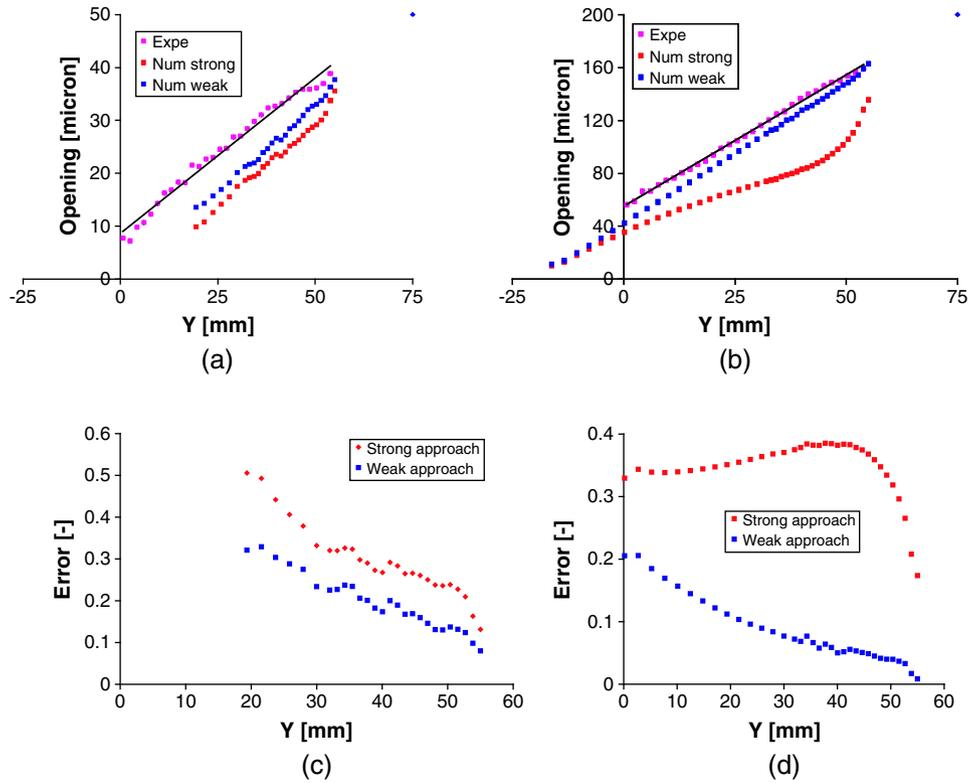
Figure 17. Comparison between strong and weak approaches versus experimental crack opening for CMOD = (a) 50  $\mu\text{m}$  and (b) 200  $\mu\text{m}$ . Corresponding errors between numerical and experimental results for CMOD = (c) 50  $\mu\text{m}$  and (d) 200  $\mu\text{m}$ .
