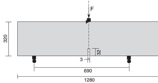
Figure 5. Three-point bending test (dimensions in millimeters).
