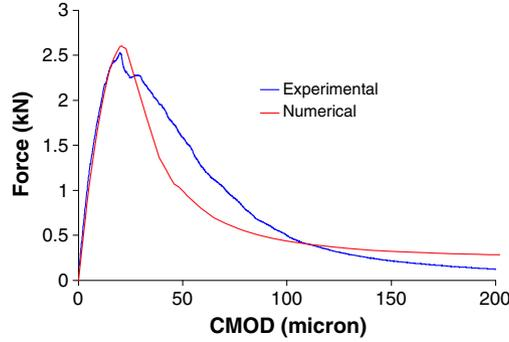
Figure 16. Experimental and numerical force versus CMOD responses.
