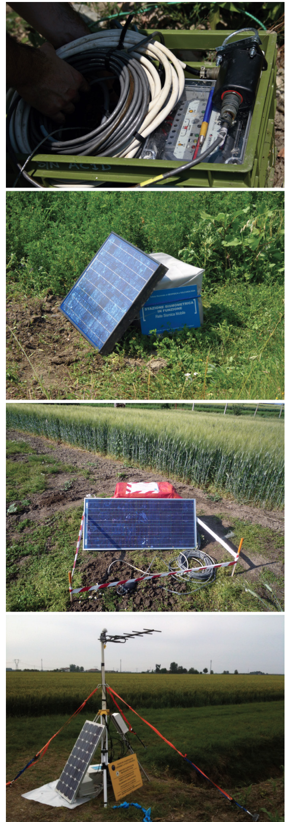
Figure 2. Photographs of the seismic deployments in the Po Plain, showing the standalone recording stations and the stations connected in real-time to the seismic monitoring center in Rome. Top to bottom: the seismic stations (digitizer, GPS, battery and cables) are transported and installed inside a plastic case. The case is covered by a tarpaulin and a sign explains the instrument scope and gives contact information. Most of the stations are powered with solar panels; the sensor is buried inside a plastic bag close to the station. Stations transmitting data in real-time are equipped with antennas.
