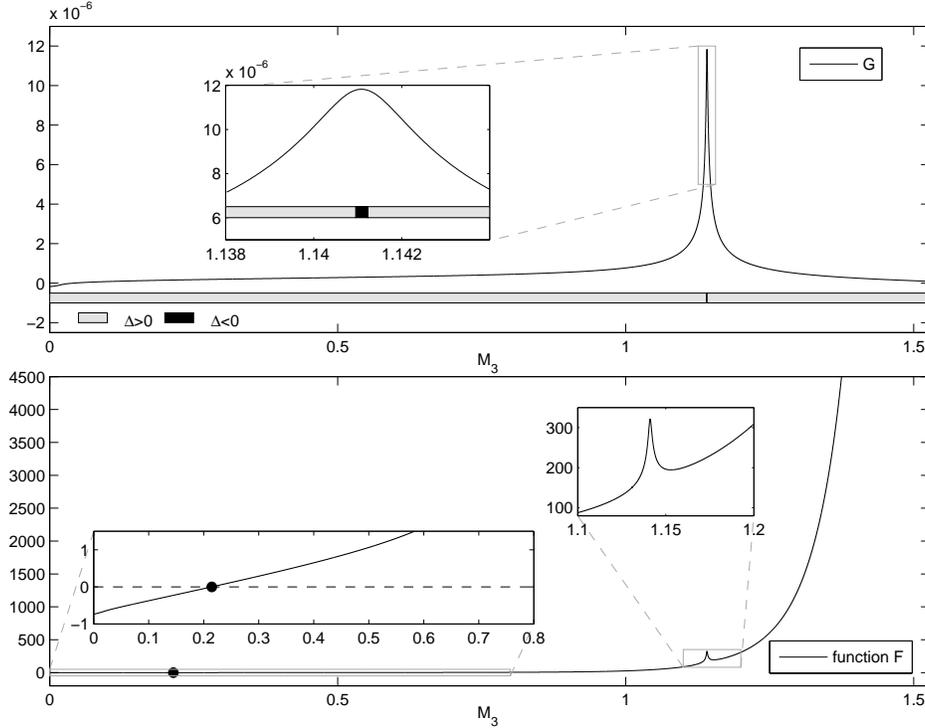
Fig. 1. Values of  $G$  (top) and  $F$  (bottom) as function of  $M_3$ , for an inlet mass flow rate of  $100 \text{ kg}\cdot\text{h}^{-1}$ , a scraper rotation speed of  $300 \text{ rpm}$  and an evaporation temperature of  $-20^\circ\text{C}$ .
