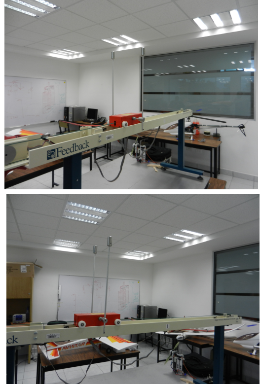
Fig 2: Inverted pendulum system used for the experiments
